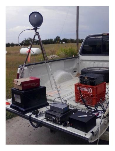
Double Balanced Mixer and 8 inch offset fed dish W5LUA worked at 13 miles Scott also heard W5RLG at 68 miles And N5WCO at 56 miles Scott has since improved his station to a larger dish plus 1 watt PA and LNA
