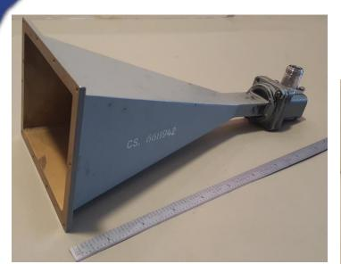
4.3" X 2.3" Horn G = 20 dBi 3dB Beamwidth ~ 17 deg
