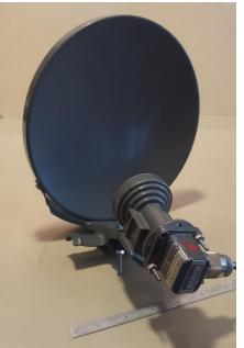
8" Offset Fed Dish G = 25 dBi 3dB Beamwidth ~ 9 deg
