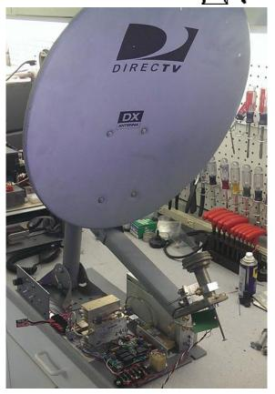
18" Offset Fed Dish G = 32 dBi 3dB Beamwidth ~ 4.3 deg
